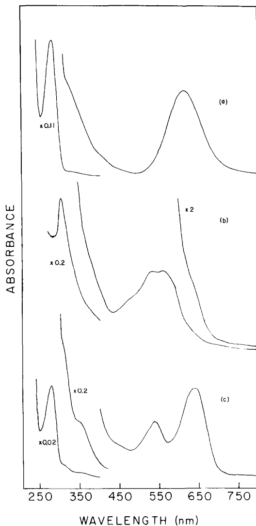
Figure 1: Absorption spectra of (a) native laccase, (0.72mM, 0-1 absorbance, 1mm cell), (b) \text{Co}^{\text{II}} -laccase run as a difference spectrum against apolaccase, (both protein solutions 0.65mM, 0-0.1 absorbance, 1mm cell), (c) \text{Co}^{\text{II}} -stellacyanin, (0.13mM, 0-0.2 absorbance, 1 cm cell), all in 25mM Tris-HCl buffer, pH 7.4.
